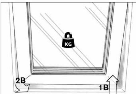
▶ **Bottomung:** Now free the sash: Lift off the sash in the hinge side (1B). Then turn the window inwards till the sash is free (2B).
