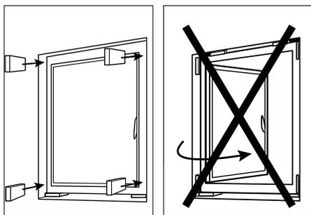
► **Do not open the window / door sash:** When only provisionally fixed with packers the window may not be opened. Before final fixing the frame may need adjustment.
