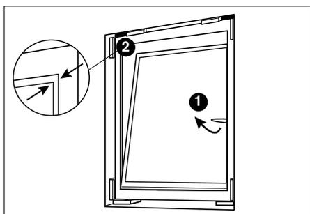
► **Pre-fixing Check Tilt Function:** With the frame securely held in the opening, carefully test the tilt function by turning the handle to the horizontal position (1).
