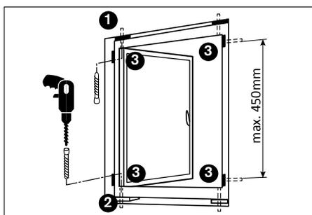
■ **Final fixing:** Install the screw no. 1 in the top frame on the hinge side as close to the side frame as possible. If this is not possible because of the brickwork, the screw must be installed in the side frame as high to the top as possible (1). Screw no. 2 is installed in the bottom frame directly below screw no. 1 (2). Fix the unit according to the current provisions as described below. Make sure that there is equal space all around the unit (3).
