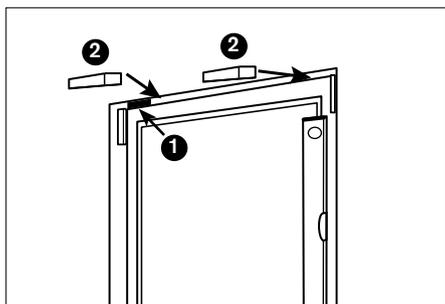
► **Support packers:** Insert fixing shims / packers at the top of the frame on the hinge side close to the corner (1). Place a wedge / air wedge on the top of the frame close to the corner in readiness for fixing the frame plumb and level (2).
