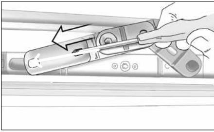
▶ **Dismounting:** Open the window/door to the tilt position. Click off the top scissor fitting: use a screw driver to lift the fitting and release it by pushing it 50mm in direction of the closing side.
