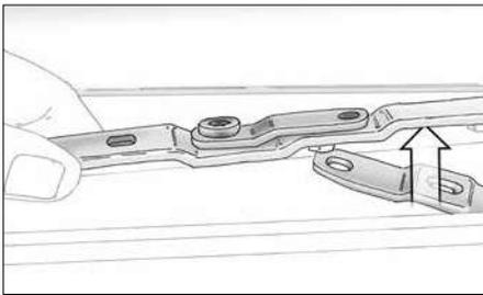
▶ Lift away the scissor fitting to disconnect sash and frame. **N.B.** When you free the sash mounting, the sash may fall out.
