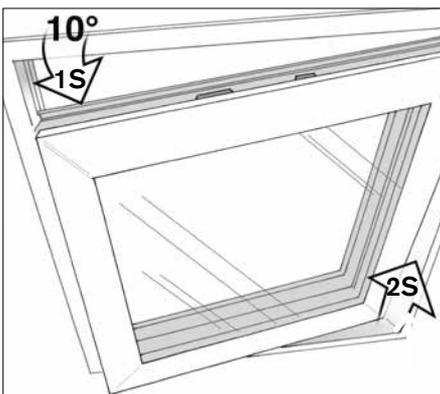
▶ **Sidehung:** Now free the sash: Turn the window approx. 10° inwards (1S) and lift off the sash in the hinge side (2S).
