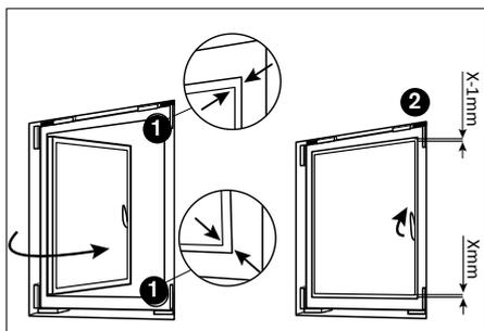
■ With the frame securely held in the opening, carefully test the turn function by turning the handle to the vertical position. When closing the window ensure that the sash rebate closes against the frame at the top and bottom corner at the same time (1). N.B. The frame must be secure within the opening.
