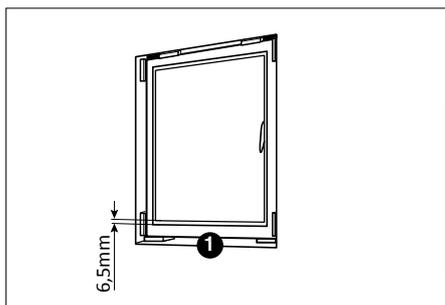
■ When the window is closed make sure there is a gap of at least 6.5mm between the sash and the frame at the bottom (1). Make adjustments if necessary.
