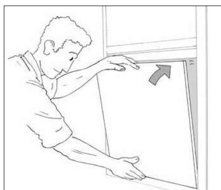
► Place the backboard in the frame and tilt it in place.
