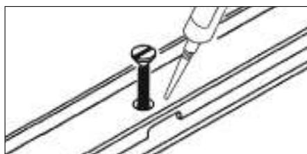
► **Adjust** the closing pressure (A) in the closing side with an open-ended spanner or adjustable wrench. Adjust the gasket pressure in the middle of the door (B).
